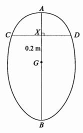
A lamina has mass 1.5 kg. Two perpendicular lines AB and CD in the lamina intersect at the point X. The centre of mass, G, of the lamina lies on AB, and XG = 0.2 m (see diagram). The moment of inertia of the lamina about AB is 0.02 kg m<sup>2</sup>, and the moment of inertia of the lamina about CD is 0.12 kg m<sup>2</sup>. The lamina is free to rotate in a vertical plane about a fixed horizontal axis perpendicular to the lamina and passing through X.
